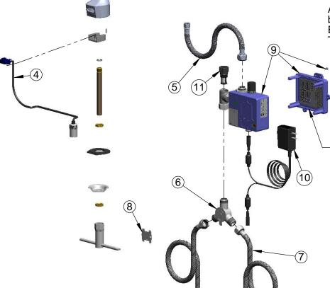
A Maximum of (8) ChekPoint Faucets can be Hardwire Connected and Powered by EC-HARDWIRE ChekPoint Hardwire AĆ Transformer. (Sold Separately)
